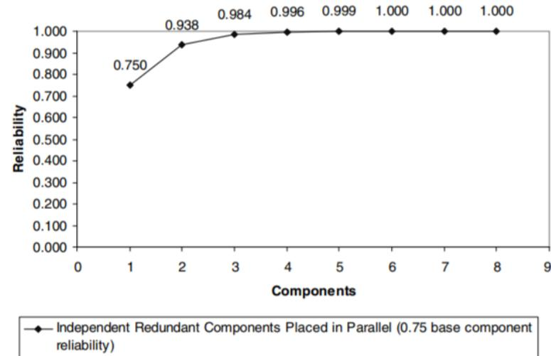
**Fig. 1.** The benefits of redundancy for reliability.
